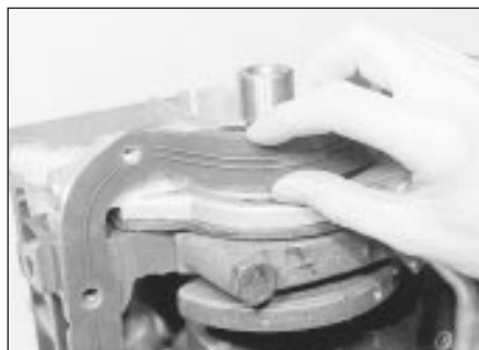
27.7 Ensure that the gasket locates correctly on the oil pump housing - 1.8 litre (R2A)
