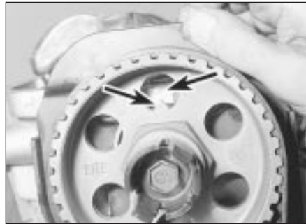
18.6b TDC pointer on camshaft sprocket aligned with dot on cylinder head - 1.8 litre (R2A)
