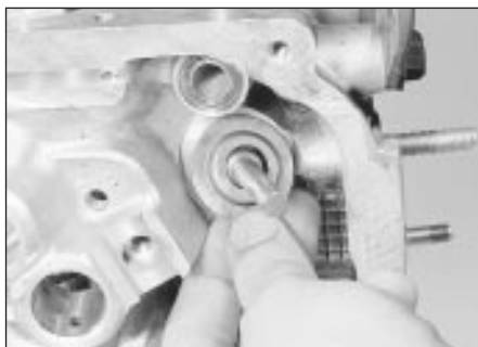
21.3a Remove the spring seat . . .
