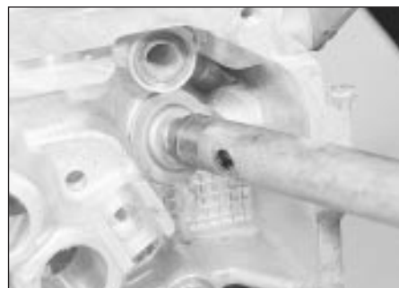
21.7 Seat each new valve seal using a metal tube - 1.8 litre (R2A)
