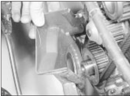
18.33c Removing the lower timing cover - 1.6/1.8 litre (R6A)
