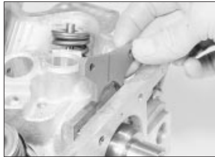
23.11a Refit the camshaft thrustplate . . .
