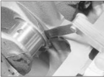
32.6 Checking crankshaft endfloat - 1.8 litre (R2A)
