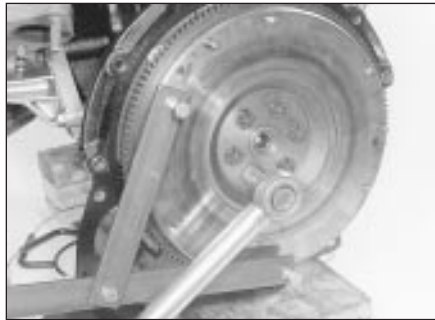
24.2 Using an improvised tool to hold the flywheel stationary while tightening the securing bolts - 1.8 litre (R2A)
