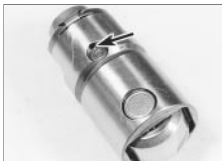
23.9a Hydraulic cam follower oil port (arrowed) - 1.8 litre (R2A)
