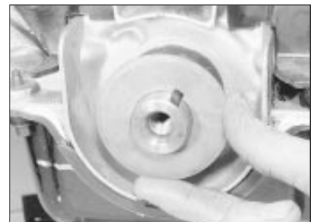
18.10c ... and the thrustwasher - 1.8 litre (R2A)
