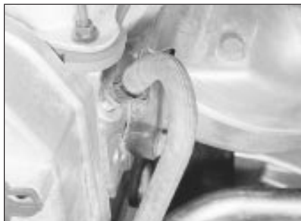
19.3b Coolant bypass hose connection at cylinder head - 1.8 litre (R2A)
