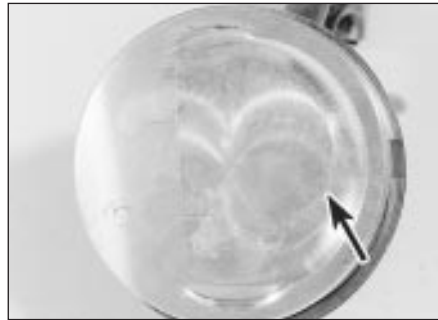
30.10a Cut-out (arrowed) in piston crown . . .
