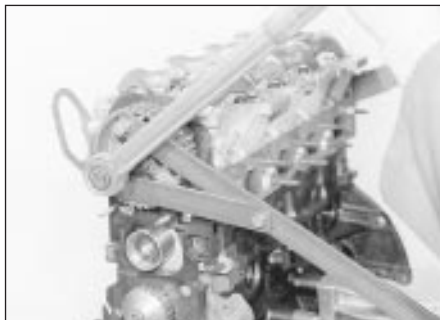
18.17 Tightening the camshaft sprocket bolt. Hold the sprocket stationary using an improvised tool with two bolts engaged in the sprocket holes - 1.8 litre (R2A)
