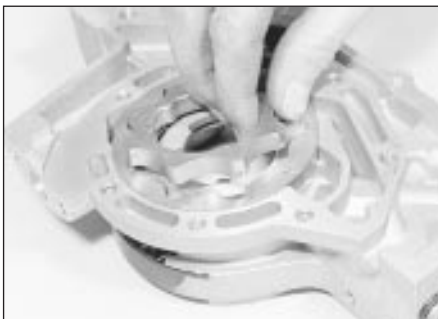
29.3 Lifting out the oil pump inner rotor
