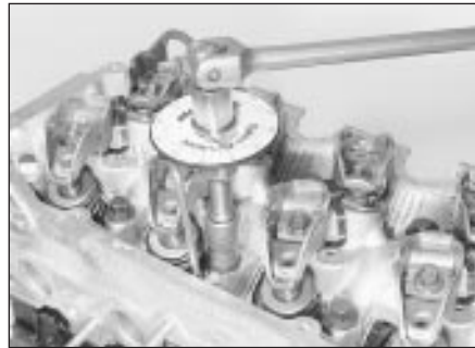
20.13b Tighten the cylinder head bolts using an angle gauge - 1.8 litre (R2A)
