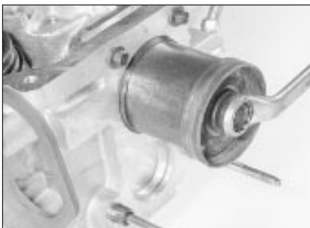
23.14 Using a special tool to fit the camshaft oil seal - 1.8 litre (R2A)
