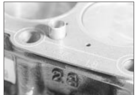
20.10b . . . then locate a new gasket with the red sealing bead and "1.8" mark uppermost - 1.8 litre (R2A)
