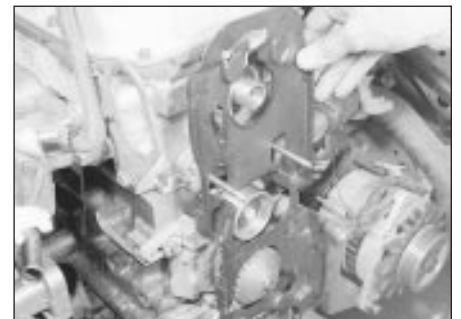
18.13 Removing the timing belt backplate - 1.8 litre (R2A)
